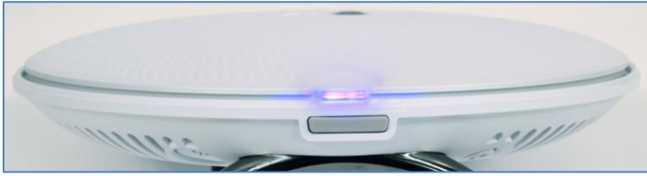
Figure 4: Purple LED – Booster is syncing
