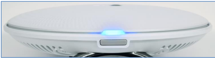
Figure 5: Blue LED – sync is complete
