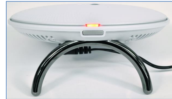
Figure 2: Red LED – Booster is ready for configuration
