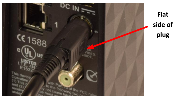
Figure 10: Aligning the power cord connector
