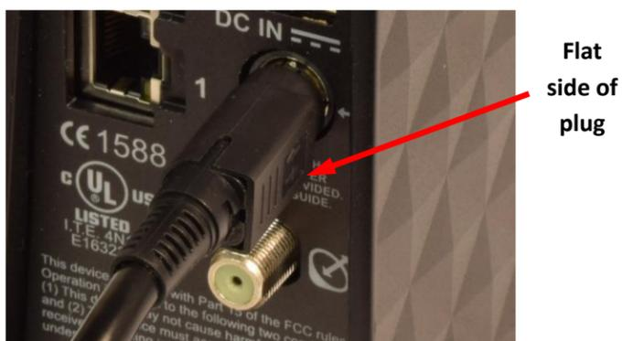
Figure 10: Aligning the power cord connector
