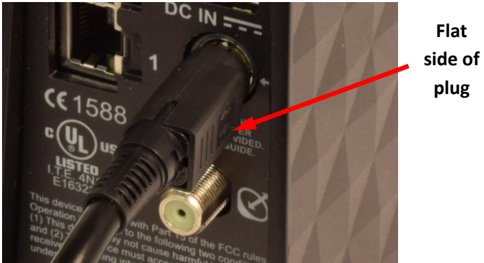
Figure 3: Aligning the power cord connector
